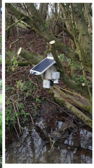
Our //Smart:River web connected, low cost, DIY sensors are monitoring the contribution of leaky dams, retention ponds and conservation agriculture to flood mitigation at sites throughout England
